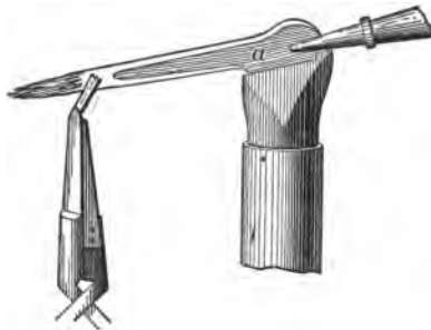
FIG. 4.—Testing fusibility, showing maximum size of fragment, manner of holding it, and position in the flame.
